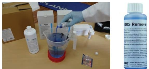
Prepare the blue liquid BRS® REMOVER in the same way as previously prepared BRS® PRECLEANER, using same water temperature (always checked with thermometer) and same amount of water (**2L**).
