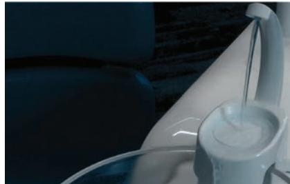
Fill clean bottle with the warm clean water (**min 40 deg.C**) and run the water through all the hoses, until all solutions are completely flushed out and the water looks clear. Do not forget about the spittoon!
