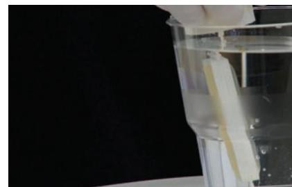
Dip the gel culture medium completely into the cup of collected water and keep it there for **10 seconds**.
