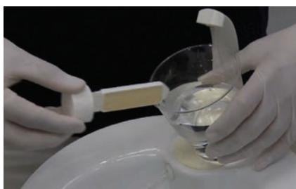
Remove the dip slide from the water and place it back into the tube.
