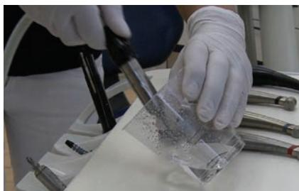
Fill a cup with a mixture of water coming from all the water lines (turbines, contra-angles, handpieces, scalers, triplex syringes and spittoon)
